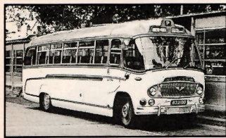
Note the special dome fitted to this Bedford SB5 Duple Super Vega bought new in 1962 for service work.
